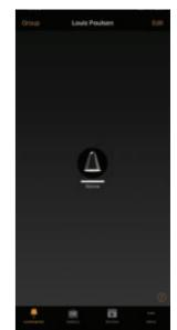
icon to turn the luminaire on or off, hold the icon and slide left or right to adjust the dimming.
