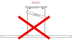
ATTENTION: Always keep the ceiling canopy horizontal when moving it and always keep the guide cables slightly taut, so that they are not damaged. Now mount the mounting box and connect the connecting cables in the lamp. Pay attention to the correct polarity when connecting the cables and connect the ground cable to the ceiling canopy again. Then push the ceiling canopy evenly and horizontally over the fixing box. The mounting is done with the magnets
