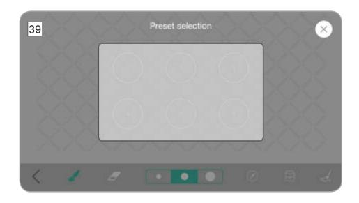
This message is displayed when pressing icon contained in screenful 37 on page 27. The page allows the user to save a layout just created as a preset. Select the desired destination by pressing on the numbered circles. If the destination is already taken by a preset, the circle background will be green. If the preset is empty, the circle background will be grey.
